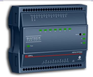
The **easy**CONTROLS EC-UV-L controller is a microprocessor-based unit ventilator controller designed to control almost any unit ventilator application. The EC-UV-L controller uses the LonTalk® communication protocol and is LONMARK certified using the unit ventilator profile #8080. The EC-UV-L is designed to work with all types of unit ventilators, including two pipe and four pipe units.
