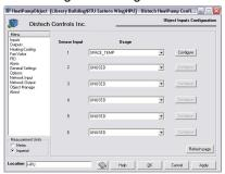
Easily configure all of the devices' parameters including inputs, outputs, fan and valve settings, heating and cooling setpoints, amongst others. You can also enable and configure additional built-in features such as optimum start, load shedding, frost protection and slave operation mode.
